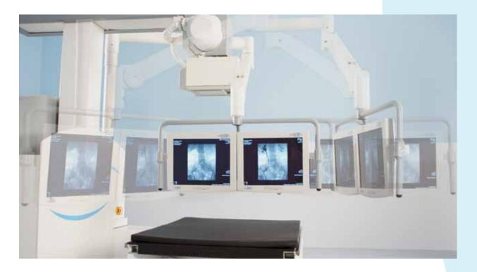
With its extended flexible articulated arm and wide range of motion, the high resolution monitors can be easily moved to either side of the table and in a variety of positions for optimal viewing.
